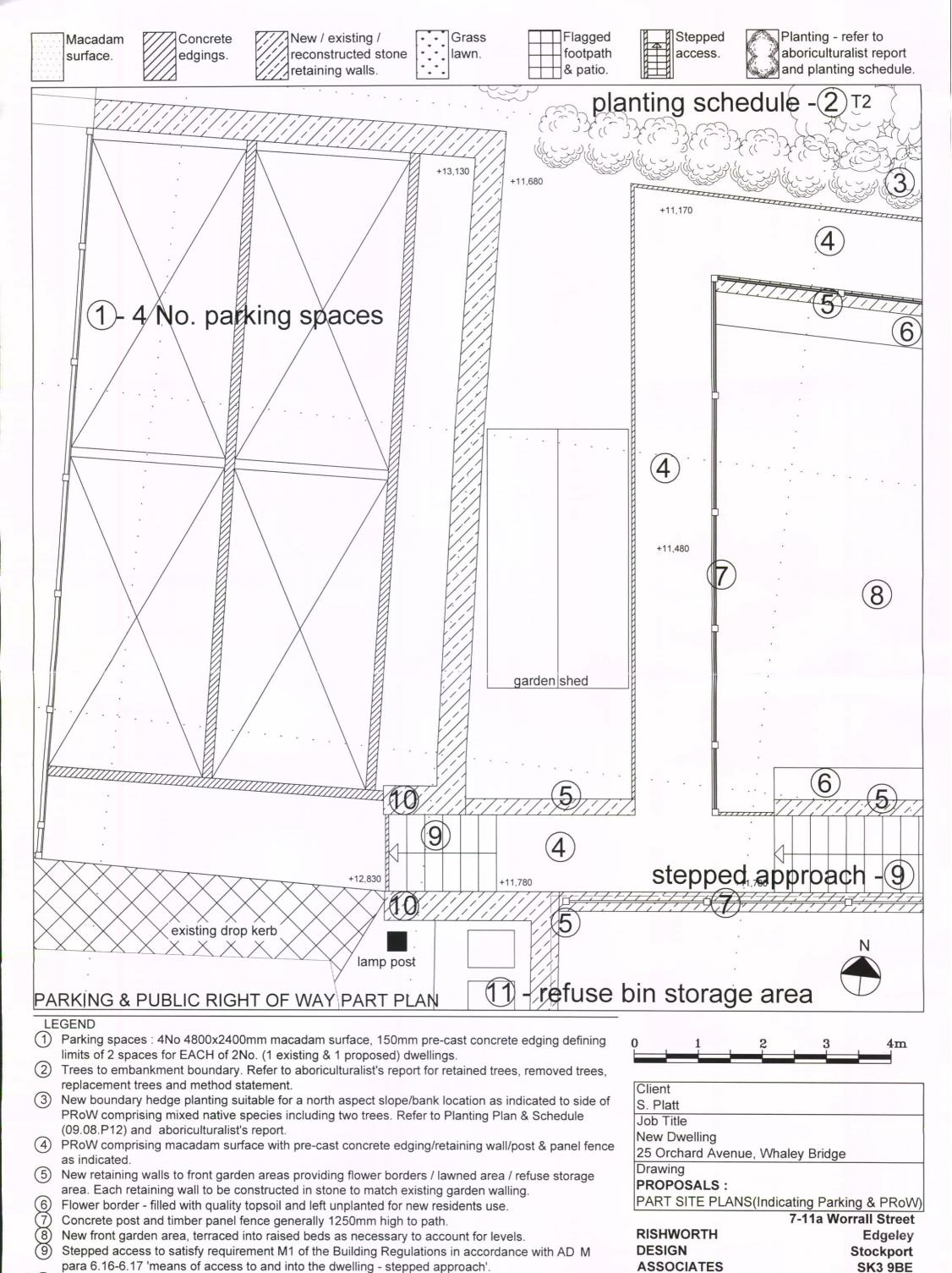
Existing retaining wall, rebuilt as necessary at PRoW access point. Provides protection to lamppost.
