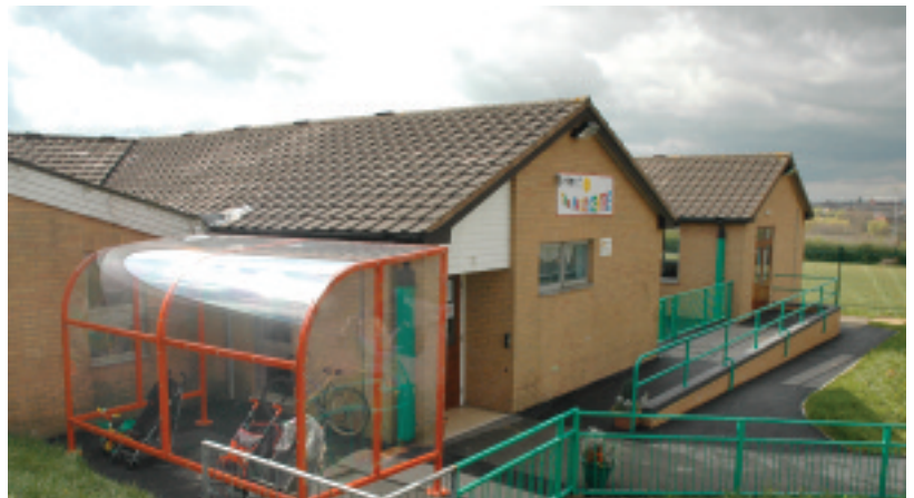
Oakhill Primary School, Tamworth. This attractive shelter is designed to securely accommodate buggies and prams. Its welded construction is tough and strong and has a number of anti-vandal features to meet today's demanding environment.
