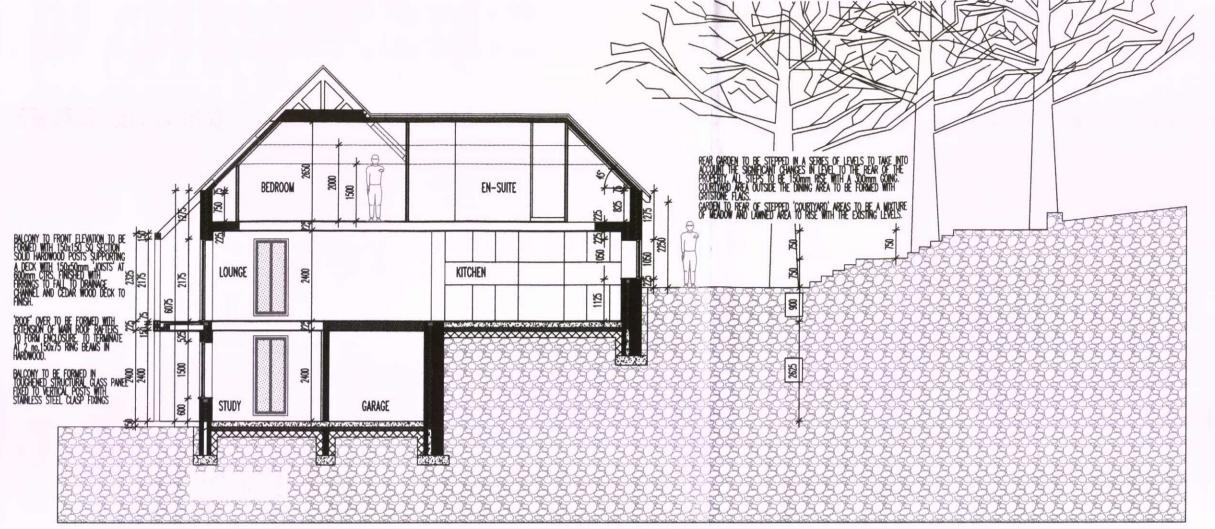
EXISTING GARAGE IS TO BE REMOVED AND THE SITE PARTIALLY EXCAVATED TO MAKE WAY FOR THE NEW DWELLING. (ALL EXISTING SITE EXCAVATED SOIL IS TO BE USED AS FILL IN OTHER AREAS TO BUILD UP LAND LEVELS.
