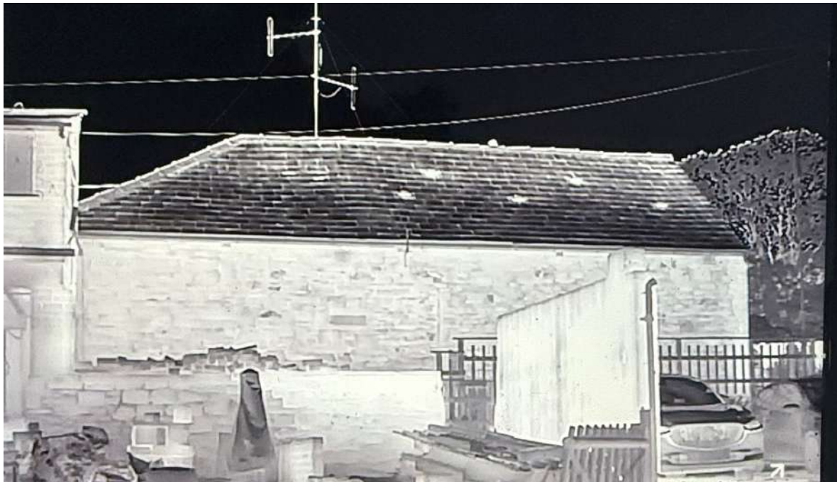
Image 4: screen shot from the thermal scope of the northern side aspect, taken during the darkest part of the night
