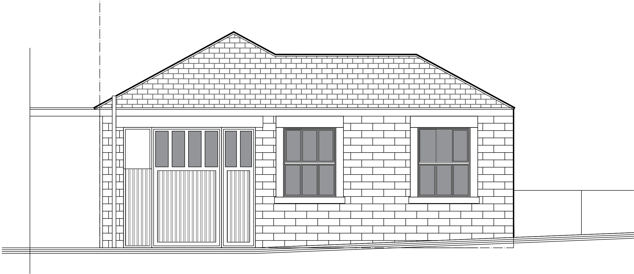
FRONT ELEVATION AS EXISTING 1:50
