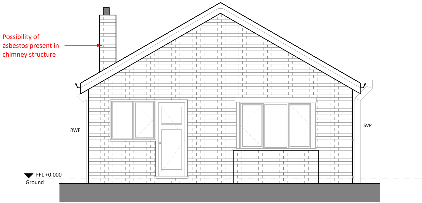
3 Rear Elevation - Existing 1 : 50
