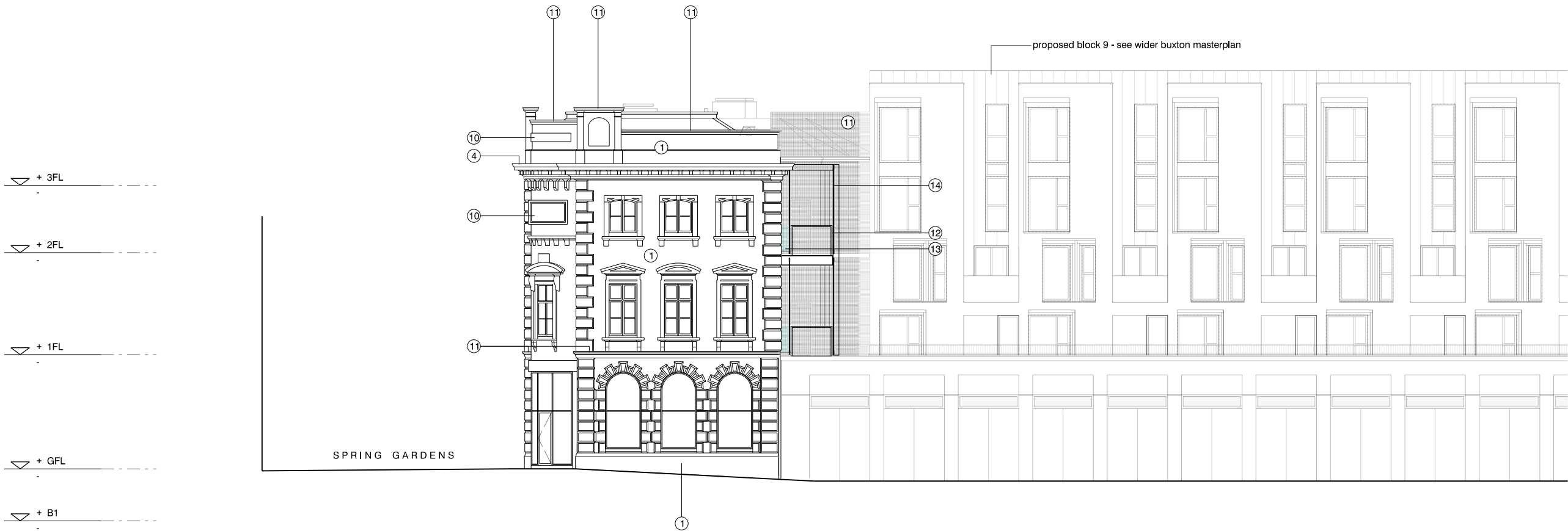
proposed repairs - elevation 04 east
