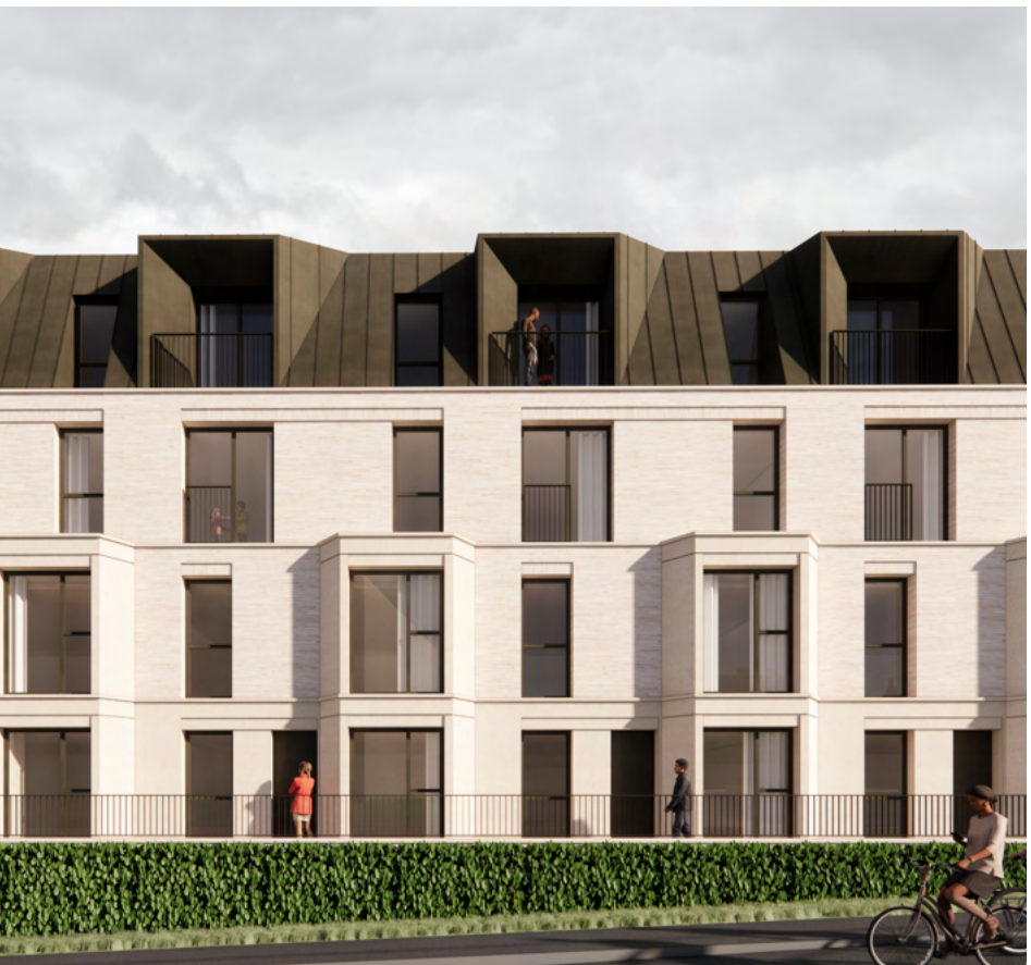
string courses, bay windows, roofscape and dormer windows
