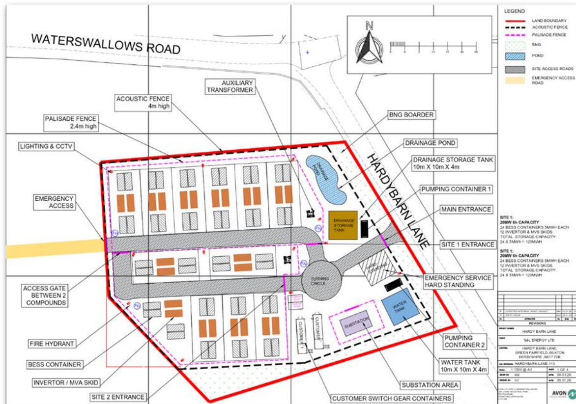
Figure 6 fire brigade facilities
