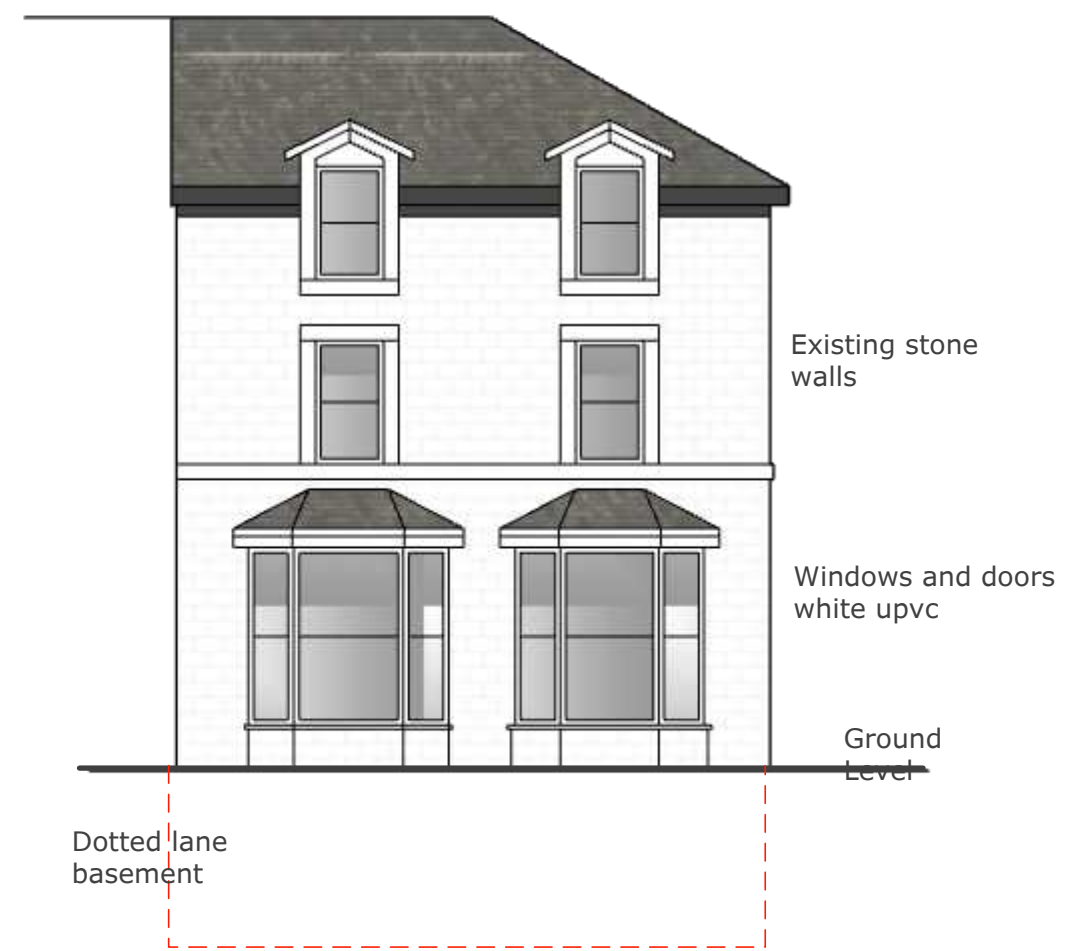
Existing Side Elevation Facing Macclesfield Road
