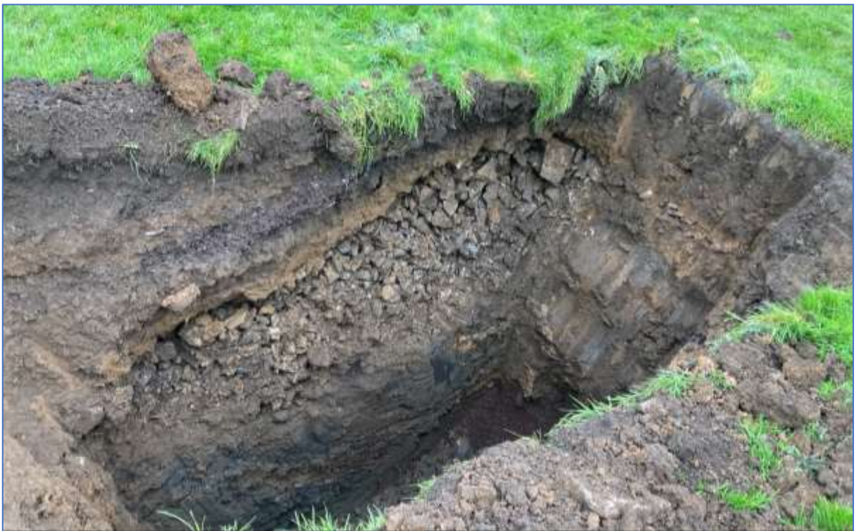
Figure 6-B: Made Ground encountered in TP108A
