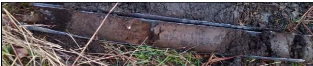
Figure 6-E: Weathered Bowland Shale Formation deposits encountered in DTS10
