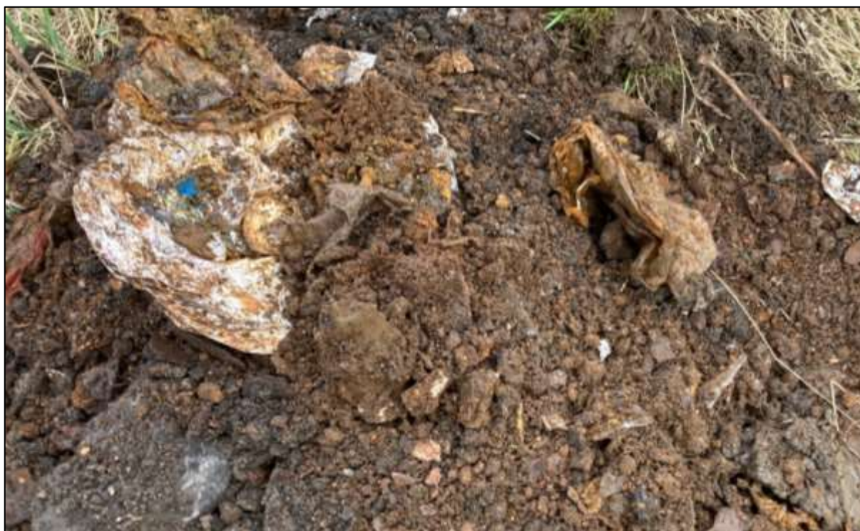
Figure 6-C: Typical Made Ground observed within the area of the proposed drainage basin
