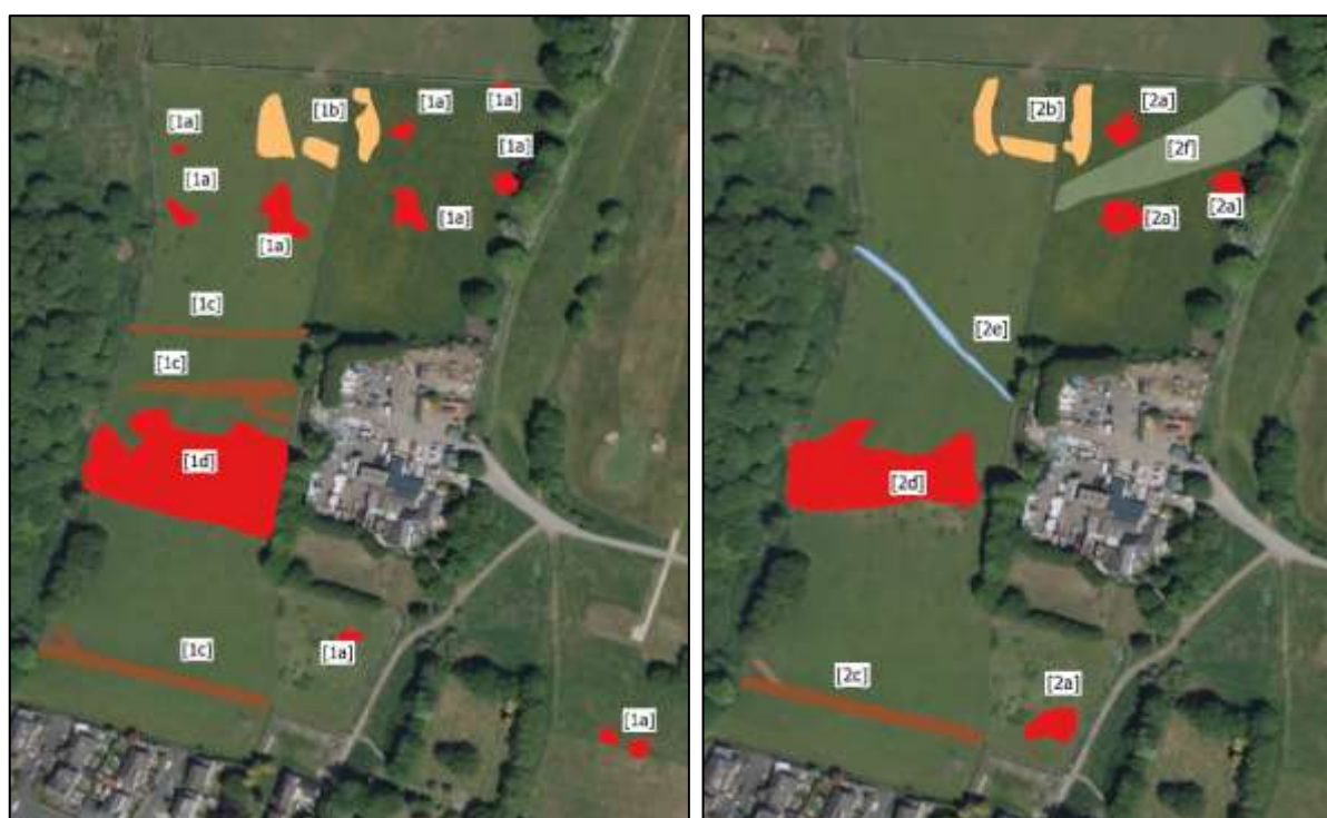
Figure 7-A: GPR responses 1a-1d (0.4-0.6m bgl) and 2a-2f (0.8-1.0m bgl)
