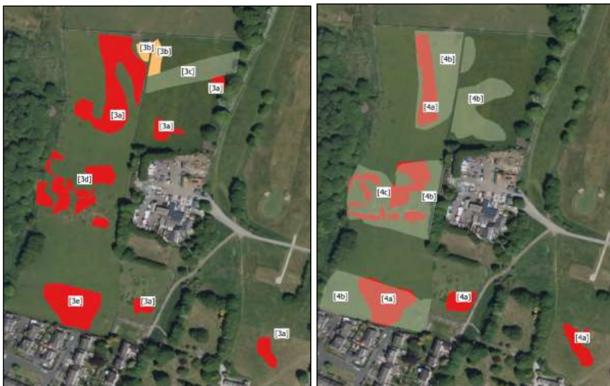
Figure 7-B: GPR responses 3a-3d (1.4-1.6m bgl) and 4a-4c (2.0-2.2m bgl)
