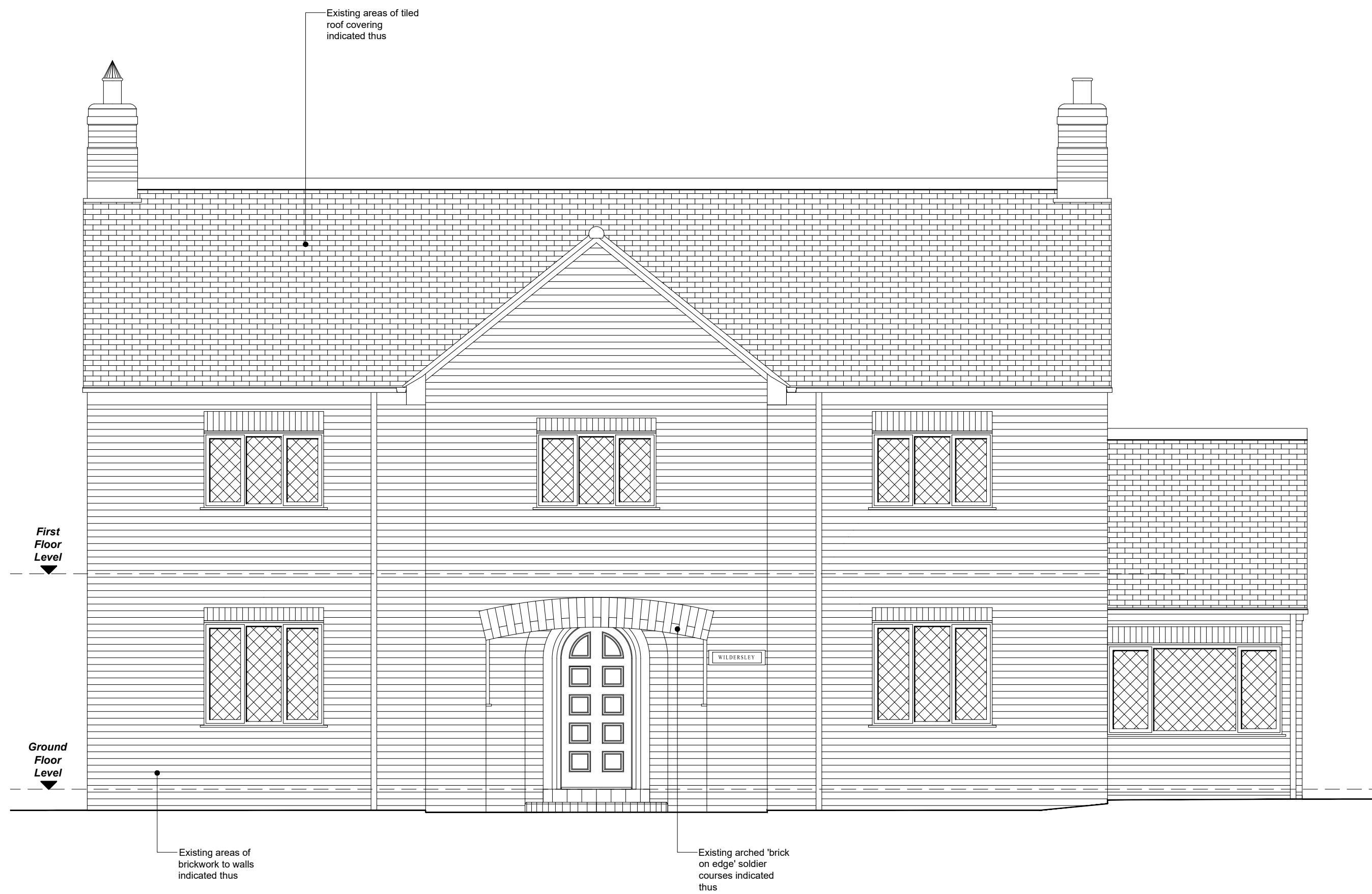
EXISTING FRONT (EASTERN) ELEVATION TO WOODHEAD ROAD
