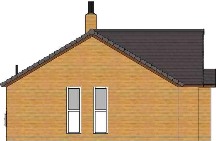
Existing Side Elevation
