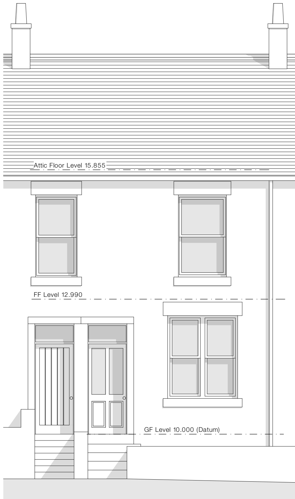
Existing North Elevation - 1:50
