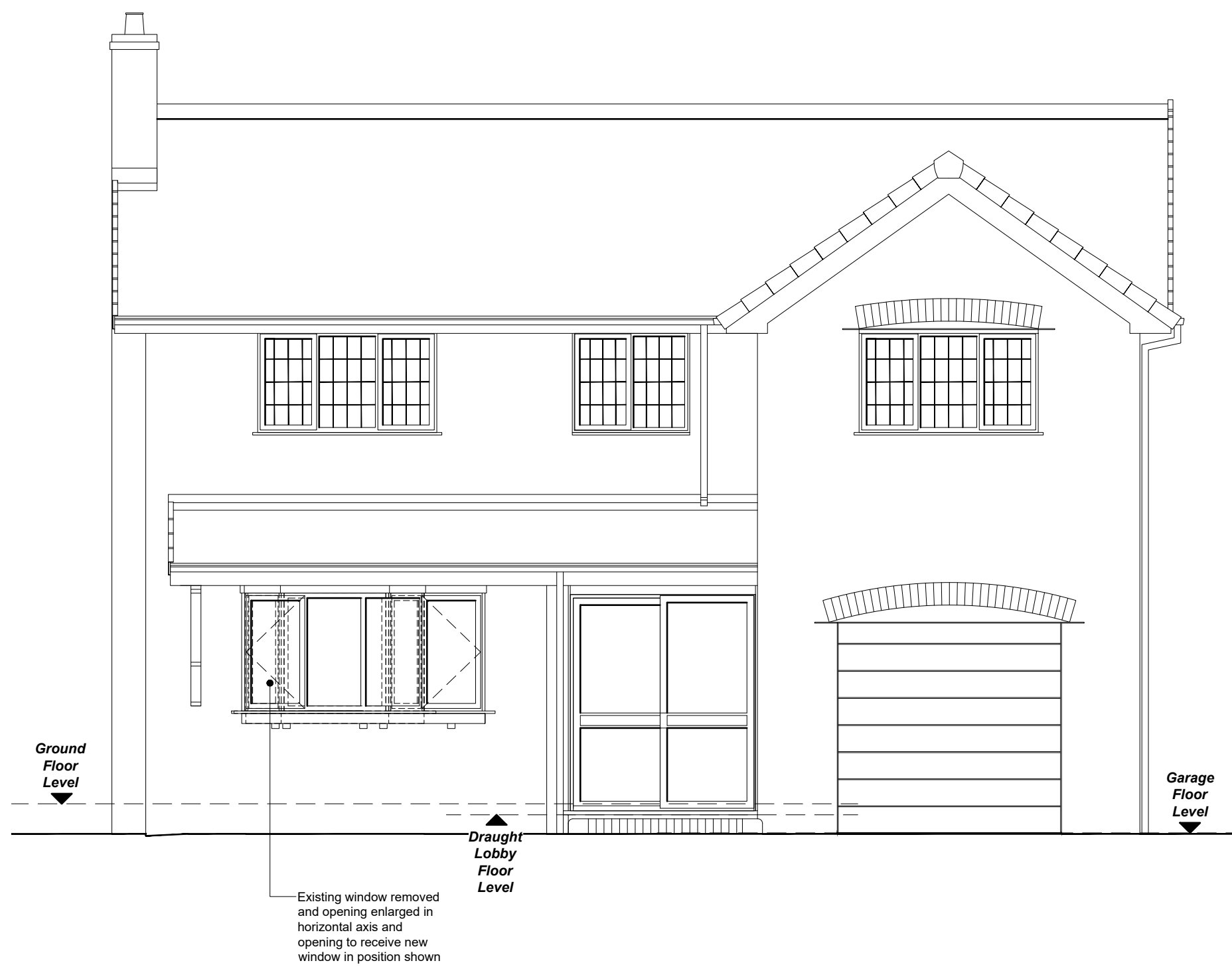
PROPOSED FRONT (WESTERN) ELEVATION TO CROFT MANOR
