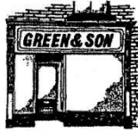
A modern fascia has been incorporated into the shopfront which is too deep and out of character with the building. The original fascia may survive underneath.
