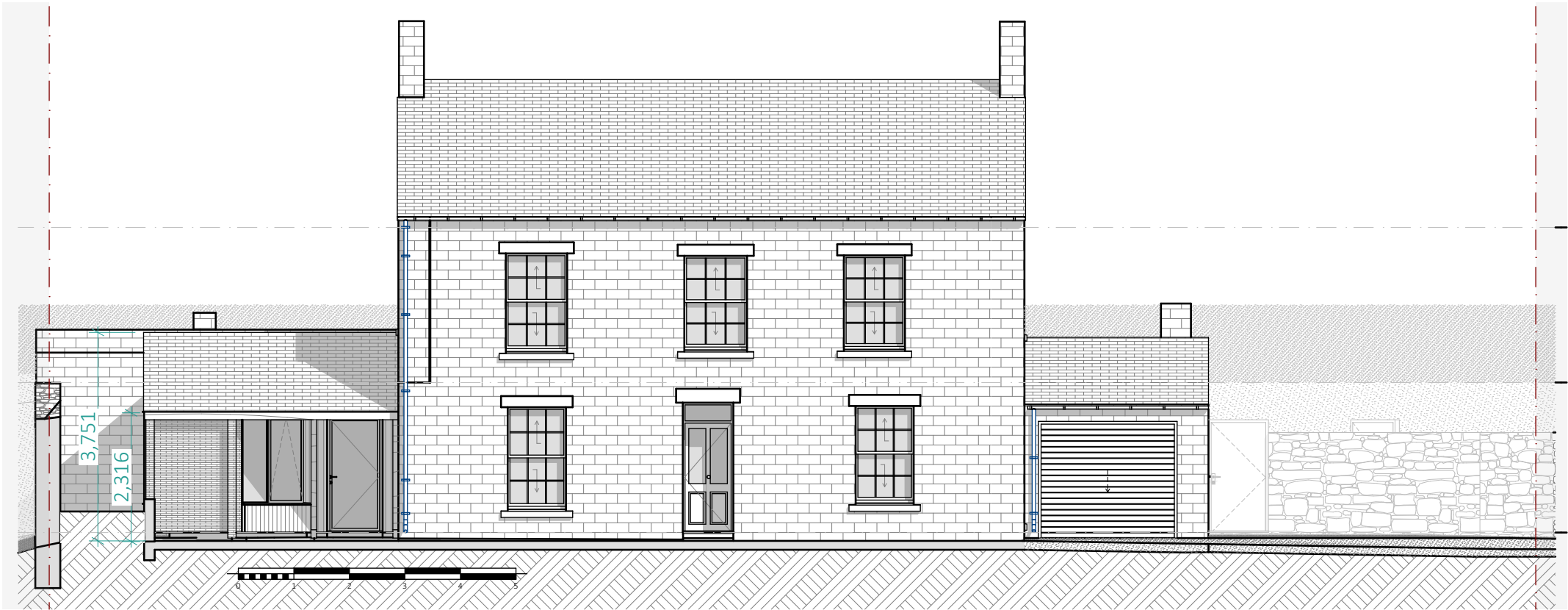
AD Elevation- South | 1:100
