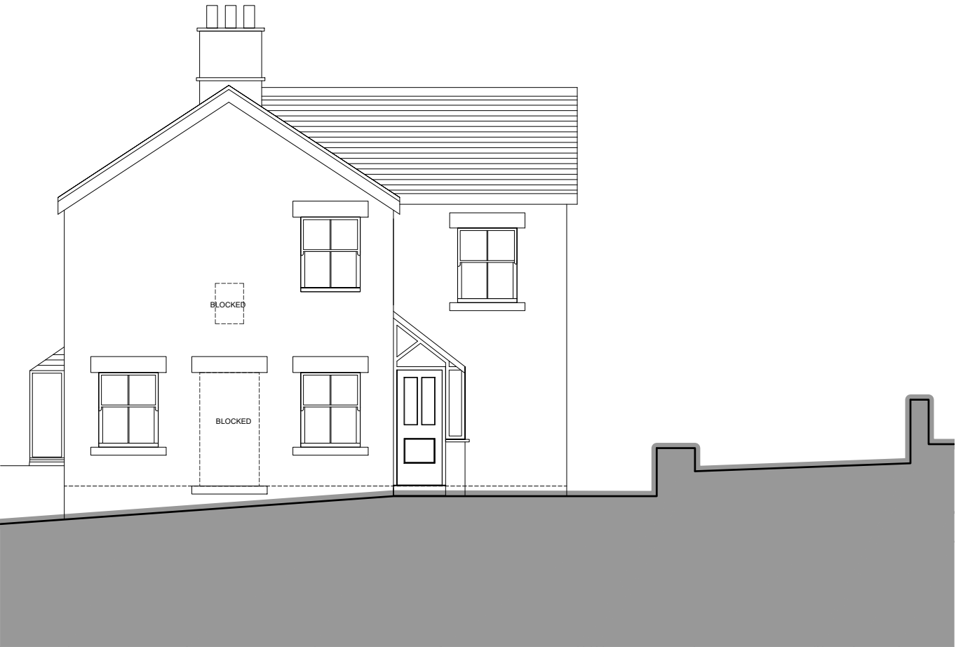
EXISTING EAST ELEVATION 1:100
