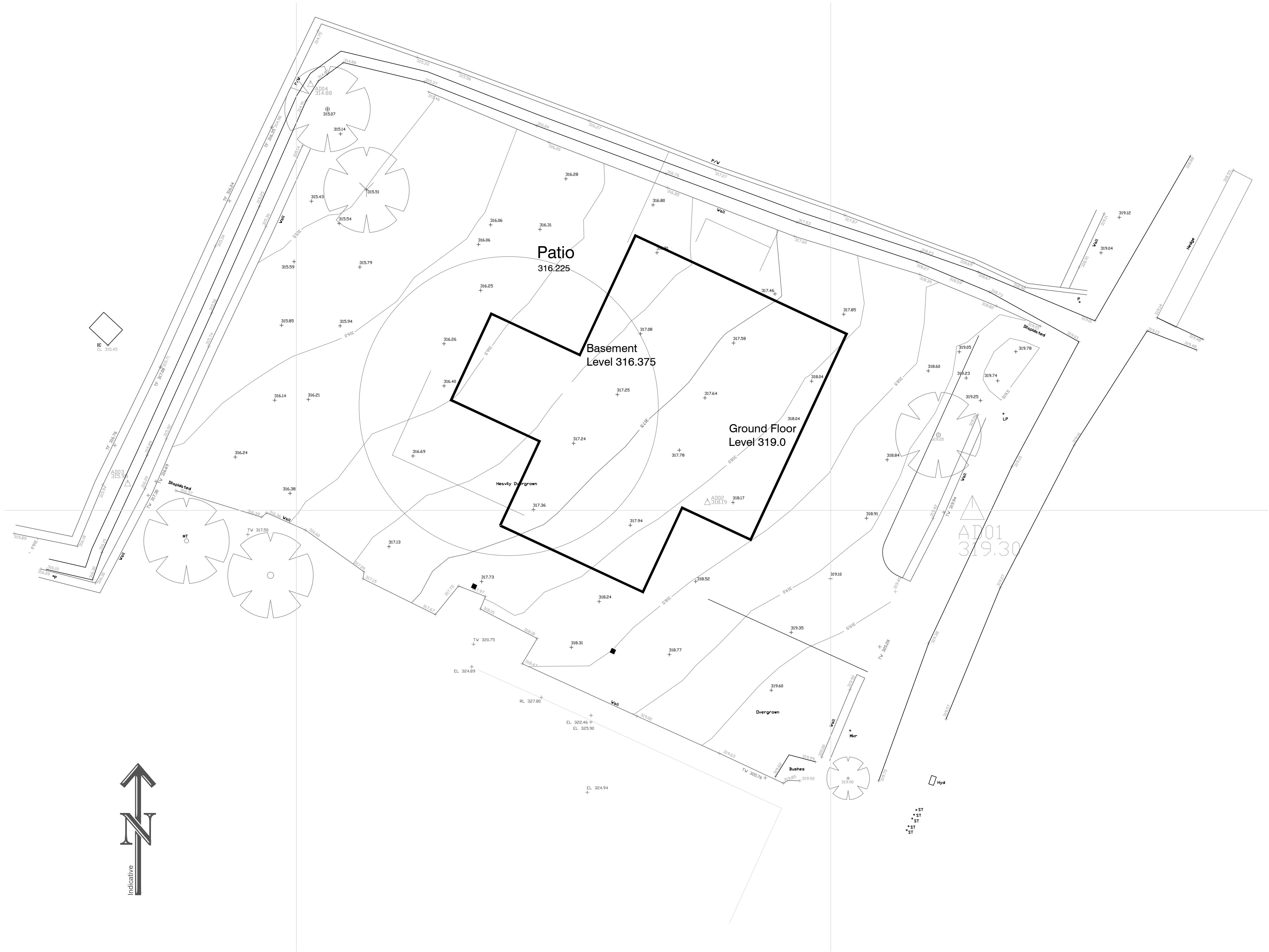
EXISTING LEVELS SURVEY WITH PROPOSED BLOCK 1:100
