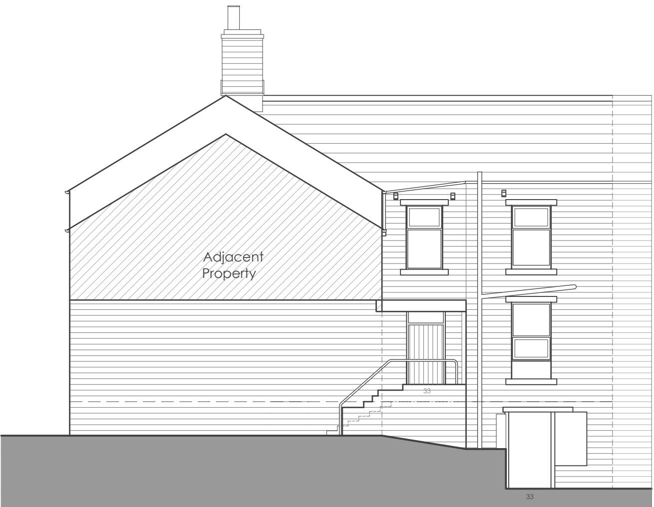
Existing Rear Elevation - Rear 1:100
