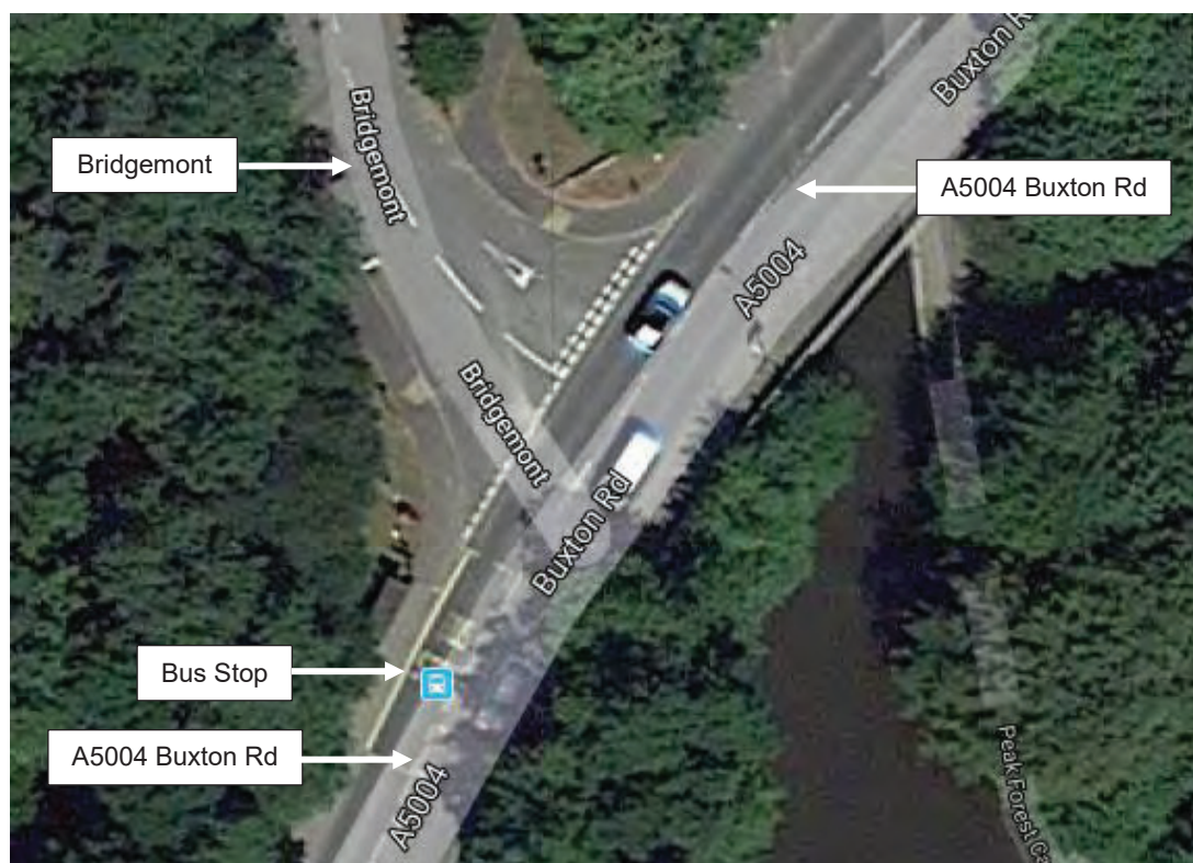
Figure 2.3 - A5004 Buxton Road/Bridgemont Priority Controlled T-Junction
