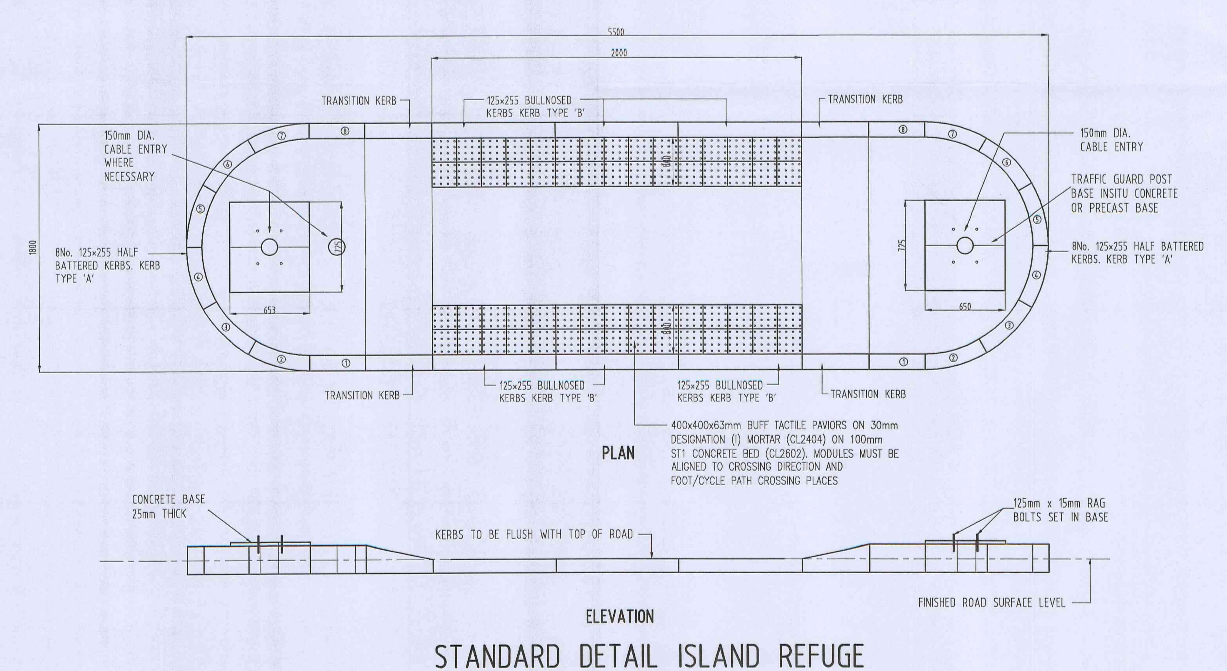
GENERAL NOTES ALL KERBS, PAVING SLABS AND CHANNELS ARE TO BE PCC TO BS 7263 : PART 1 - 1994 UNLESS NOTED OTHERWISE. CONCRETE BED AND HAUNCH TO BE STANDARD MIX - ST1 KERBS & SLABS ARE TO BE CUT USING A DISC CUTTER. DROPPER KERBS TO BE USED TO REDUCE THE KERB FACE AT VEHICLE AND PEDESTRIAN CROSSINGS.
