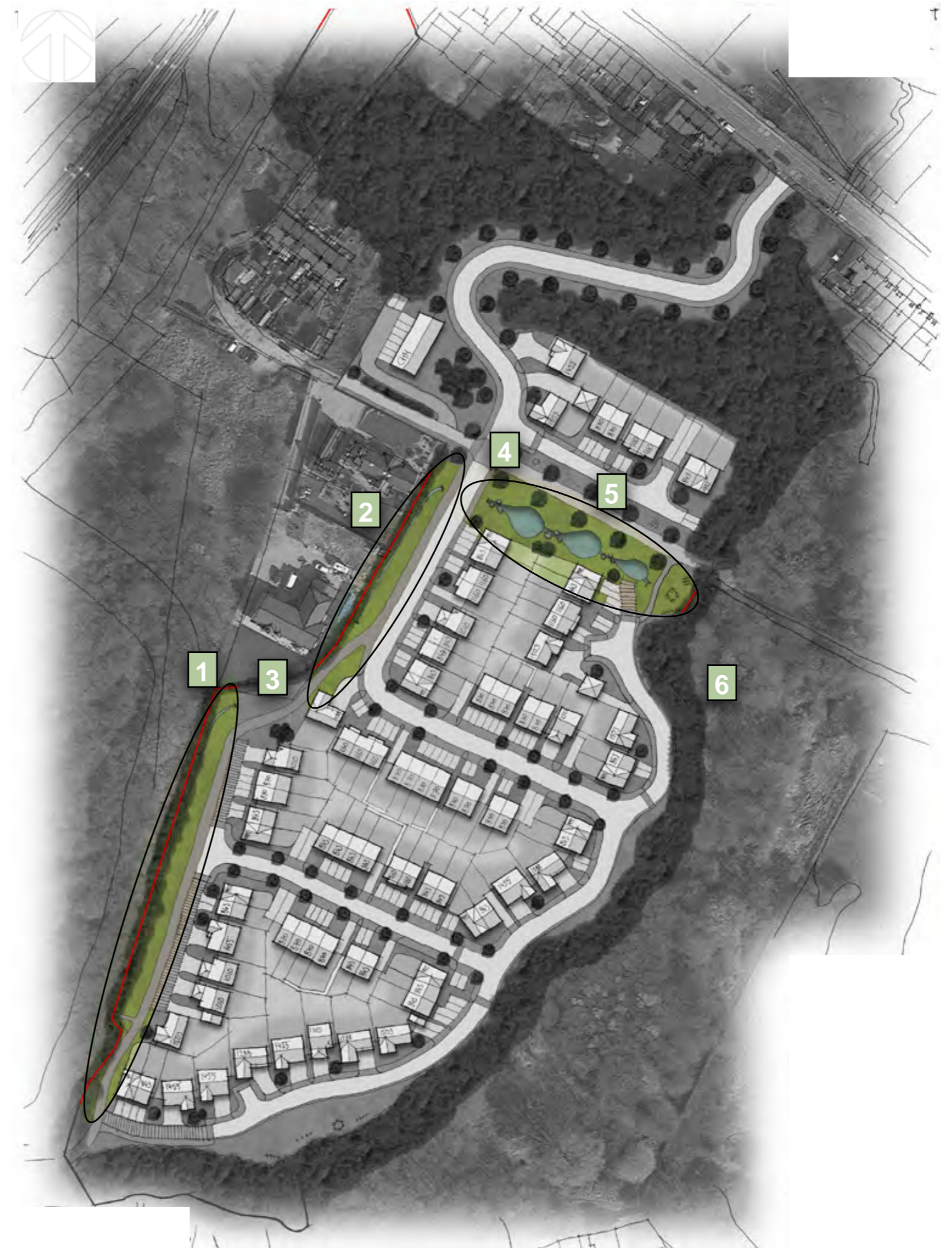
Dinting Vale Colour Layout depicting surface water drainage elements
