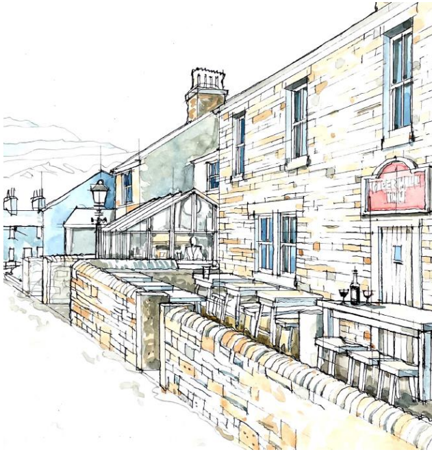
Figure 7: Artist Impressions -indicating the simplicity of design, the use of glazing to ensure link to new use and also visual link to the existing building. Maintain the scale and language of the existing building through the use of existing materials and scale.
