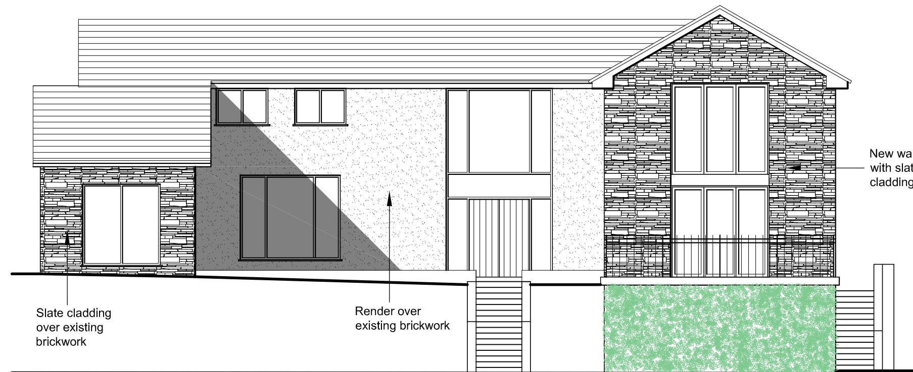
Front Elevation (South West)
