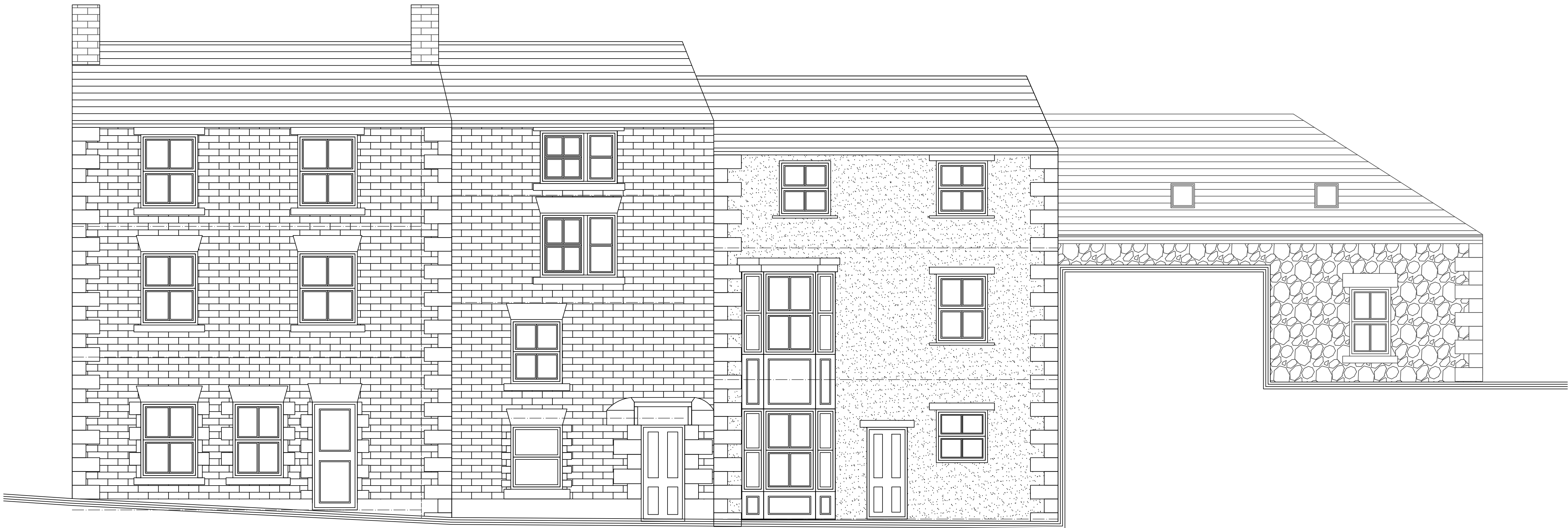
PROPOSED FRONT ELEVATION SHOWING SIDE TO BARN 1:50
