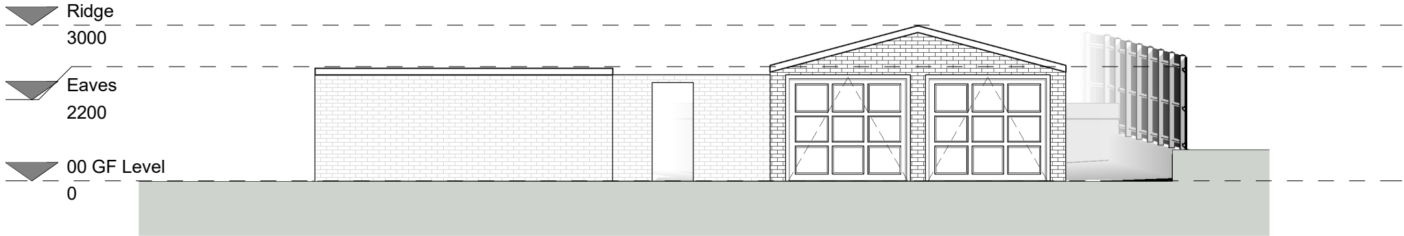
North West Elevation - Garage Only 1 : 100
