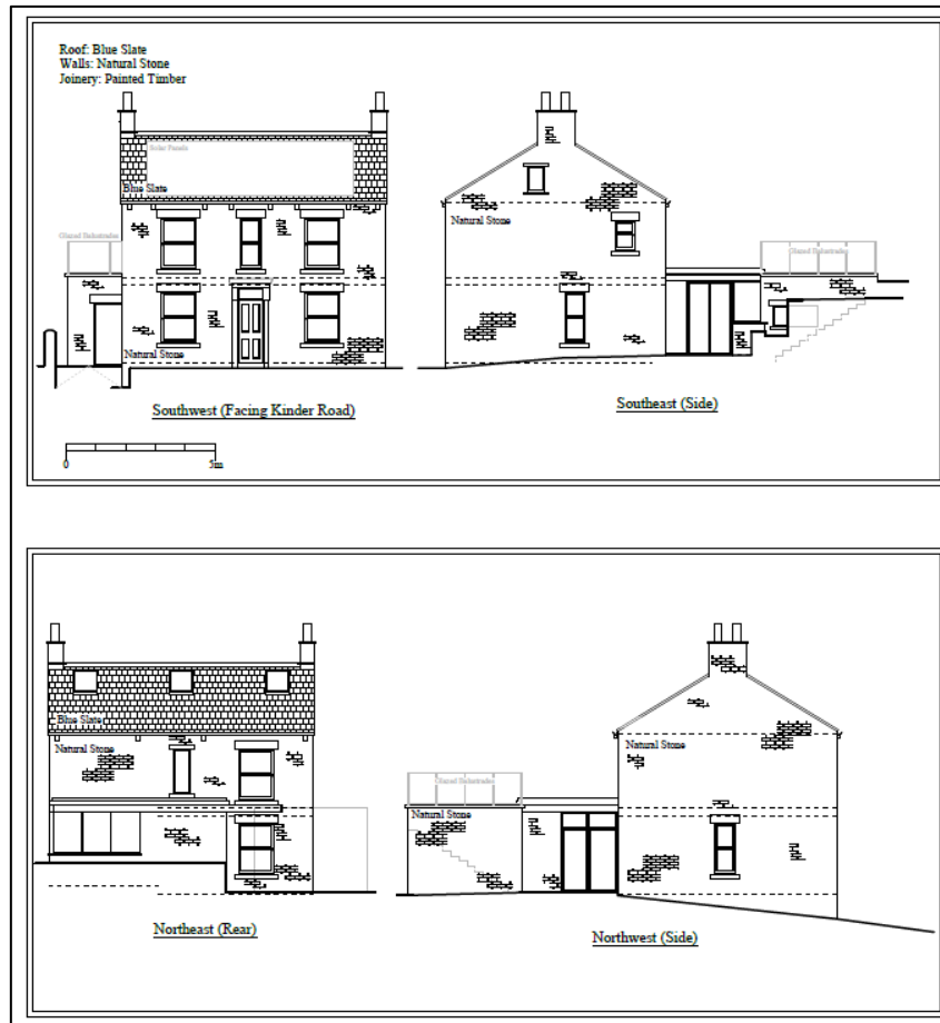
Figure 6: Elevations as Existing
