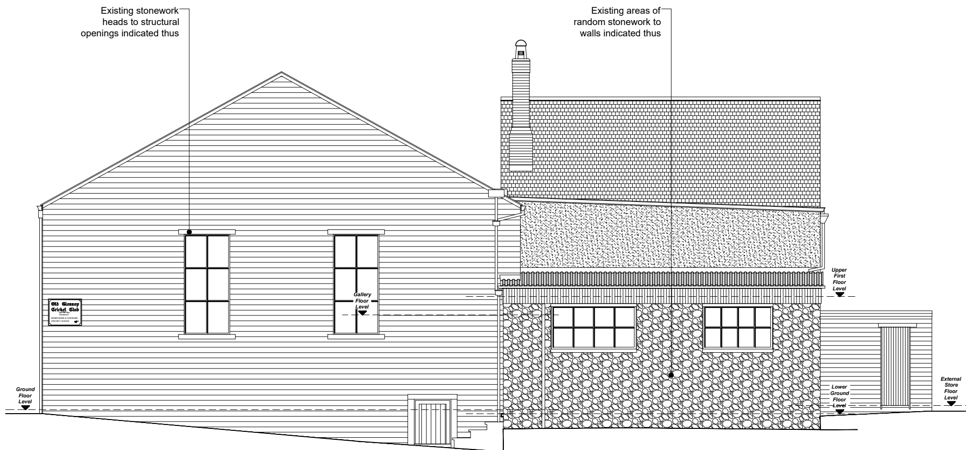
EXISTING SIDE (SOUTHERN) ELEVATION
