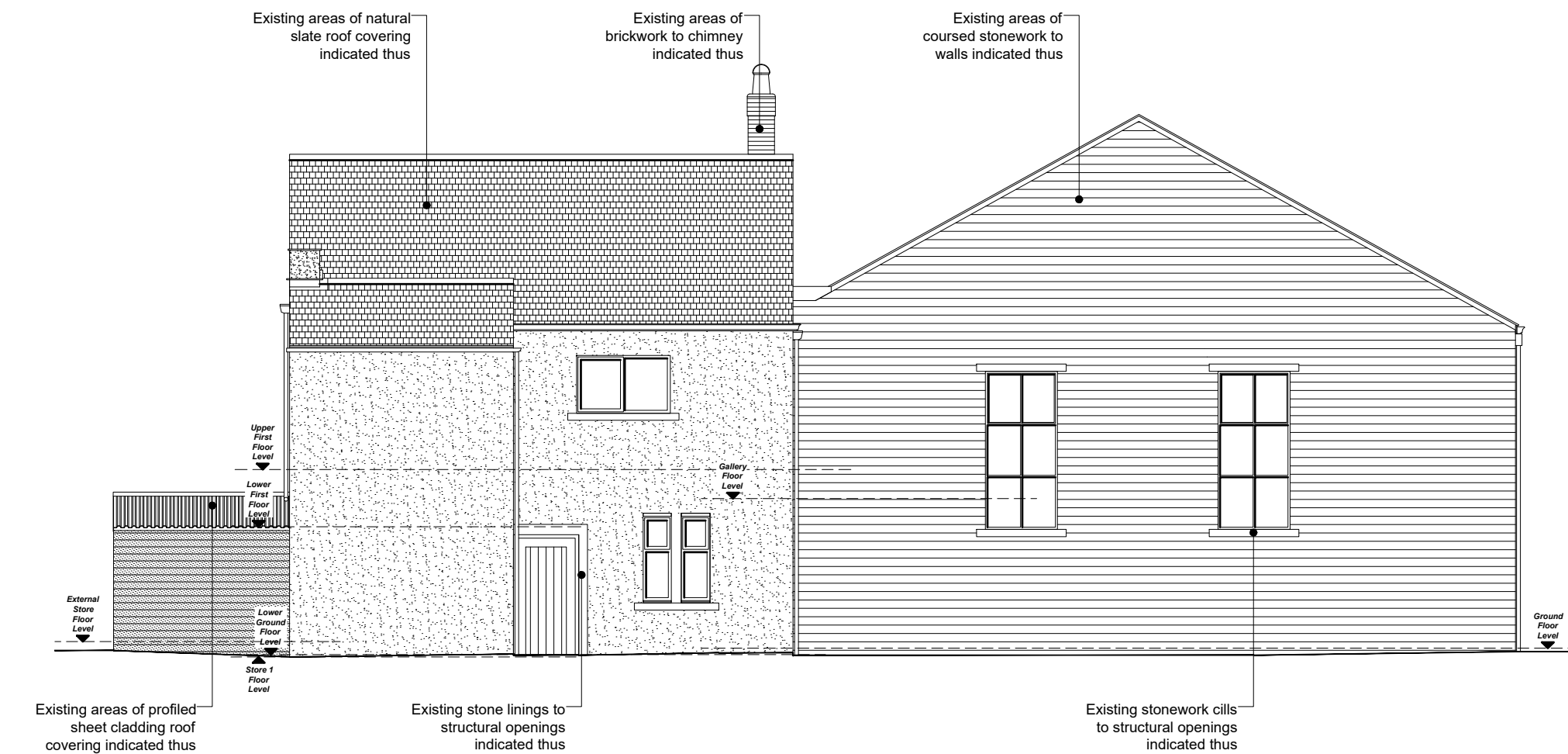
EXISTING SIDE (NORTHERN) ELEVATION
