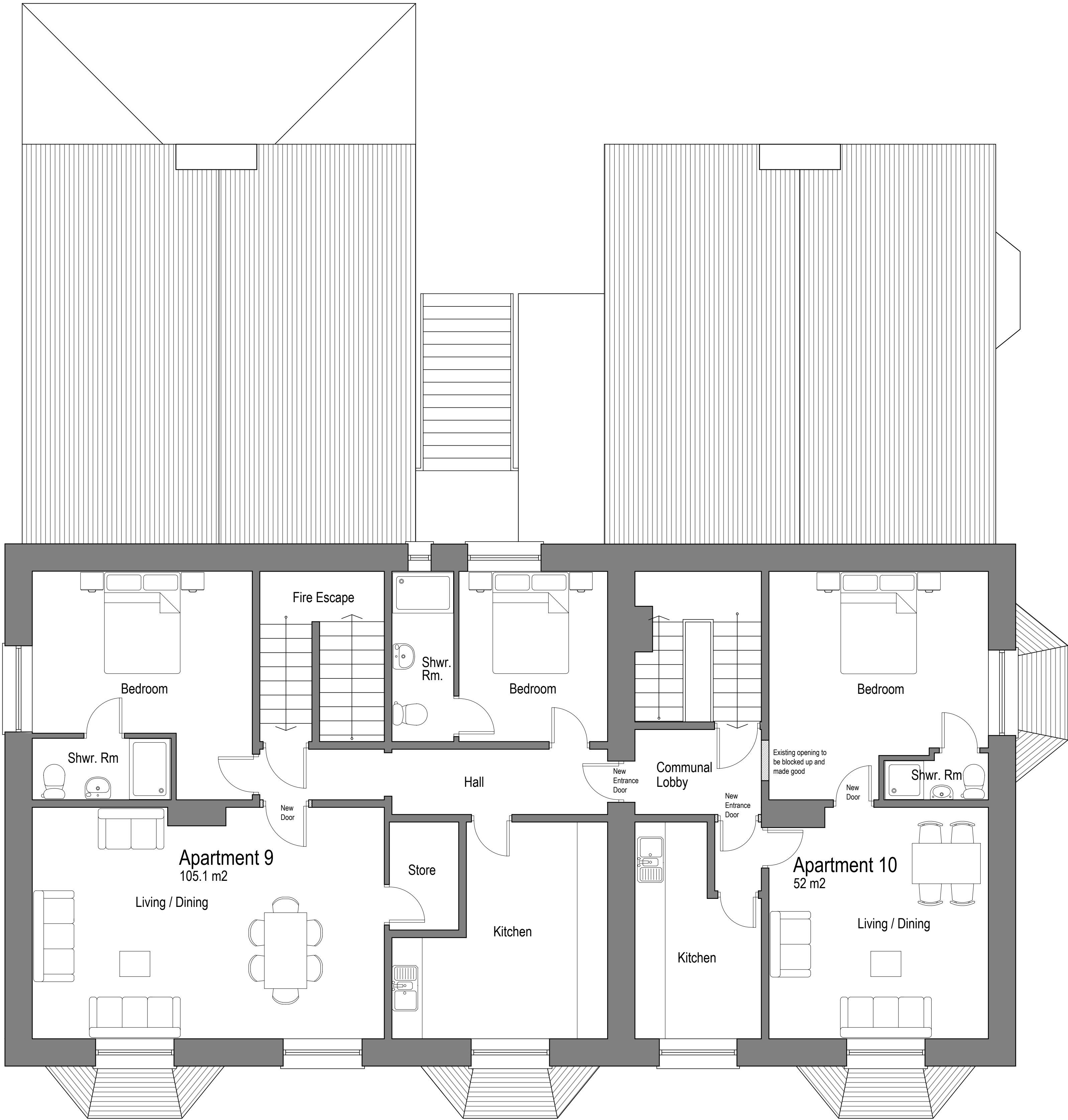
Proposed Second Floor Plan
