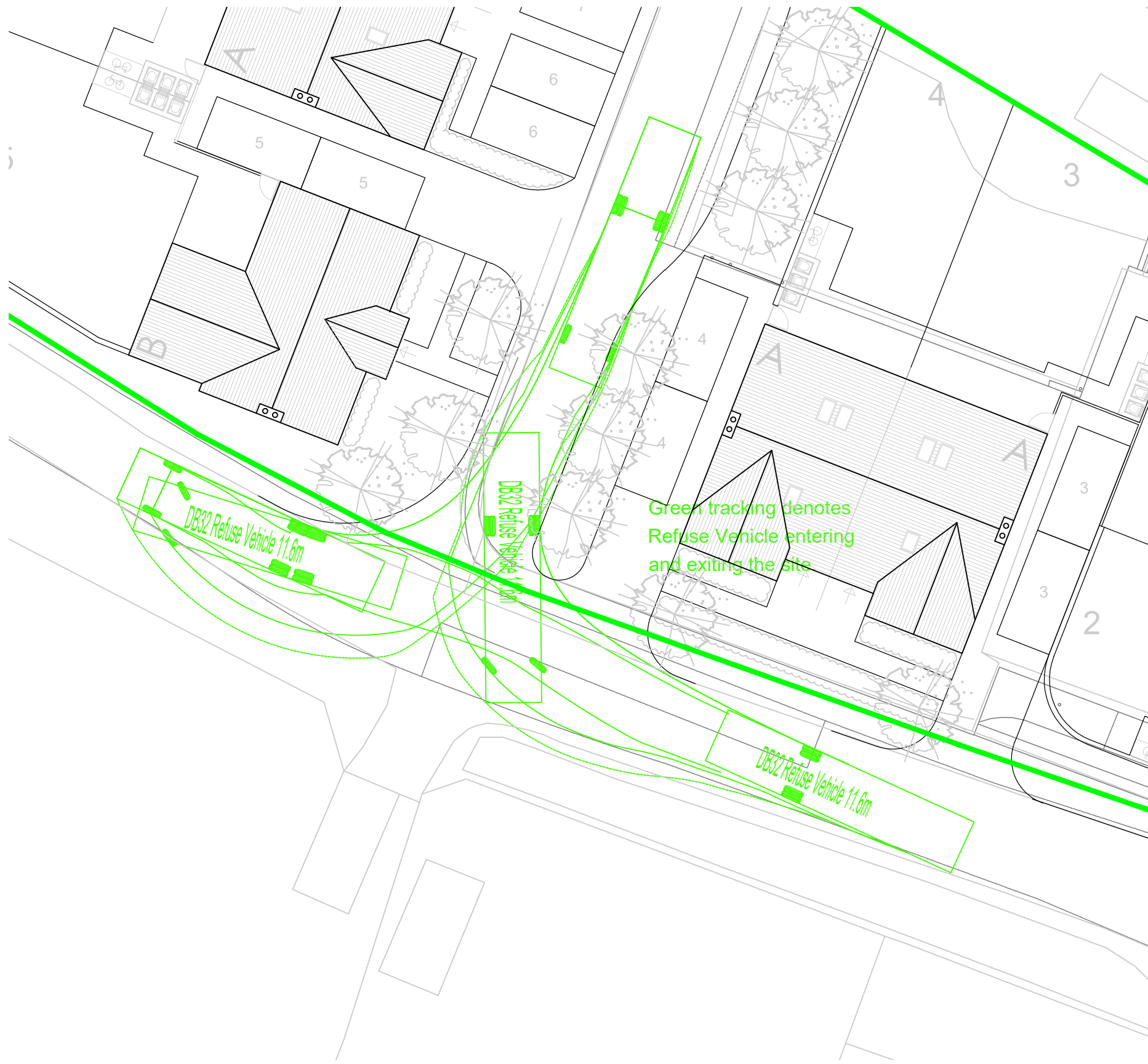
REFUSE VEHICLE TRACKING ENTERING AND EXITING THE SITE [SCALE 1:200]
