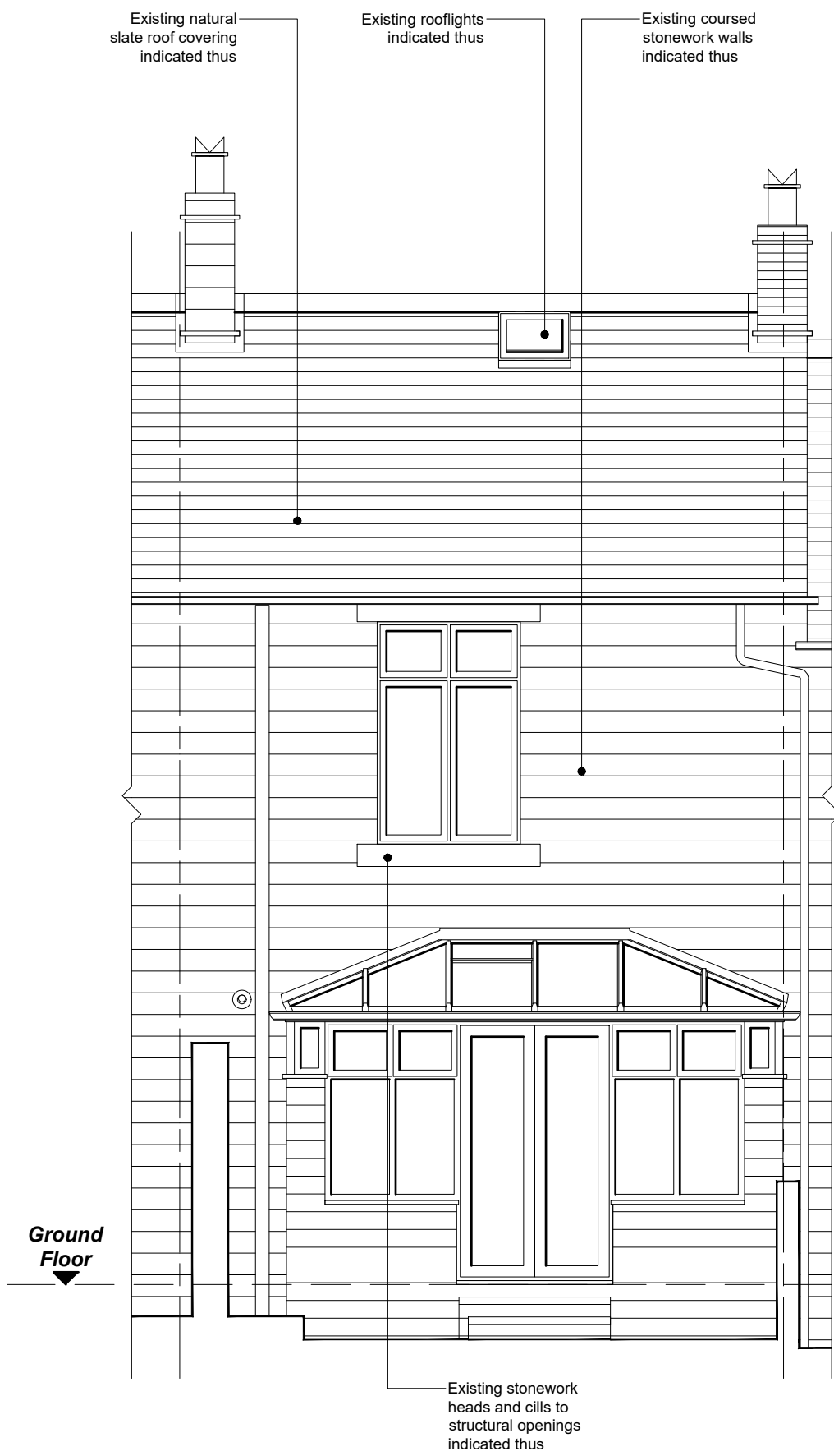
EXISTING REAR ( NORTH WESTERN) ELEVATION
