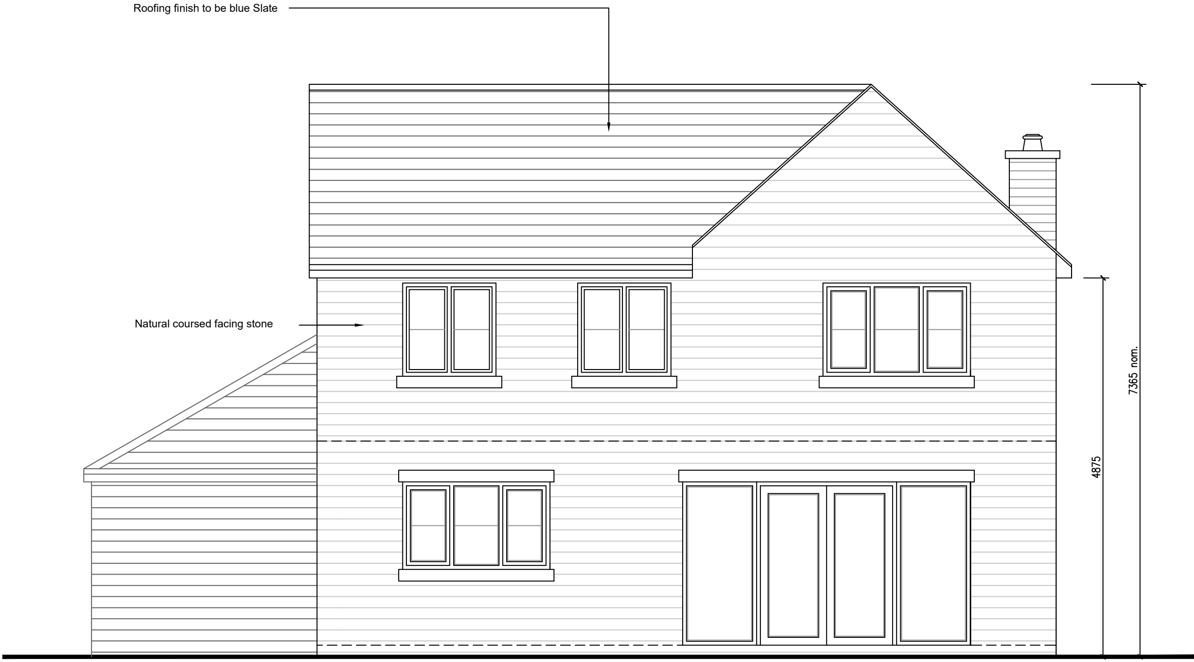
Rear Elevation as Proposed Scale @ 1 : 50
