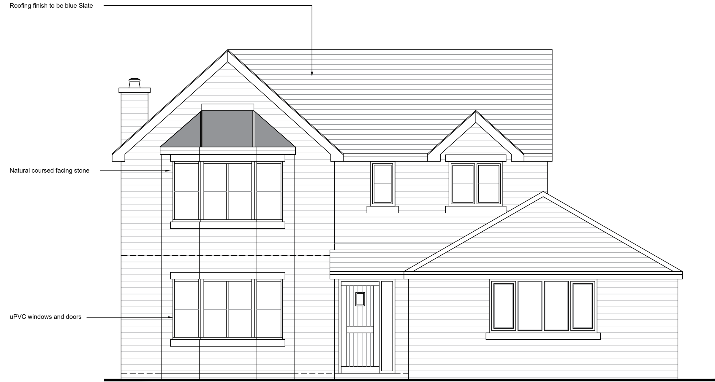
Front Elevation as Proposed Scale @ 1 : 50
