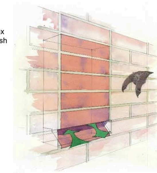
Habibat 001 Bat box built into outer skin of gable wall
