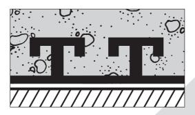
The concrete slab is cast over the laid membrane and Holdfast system. The concrete displacing itself around the 'T' bar sections.
