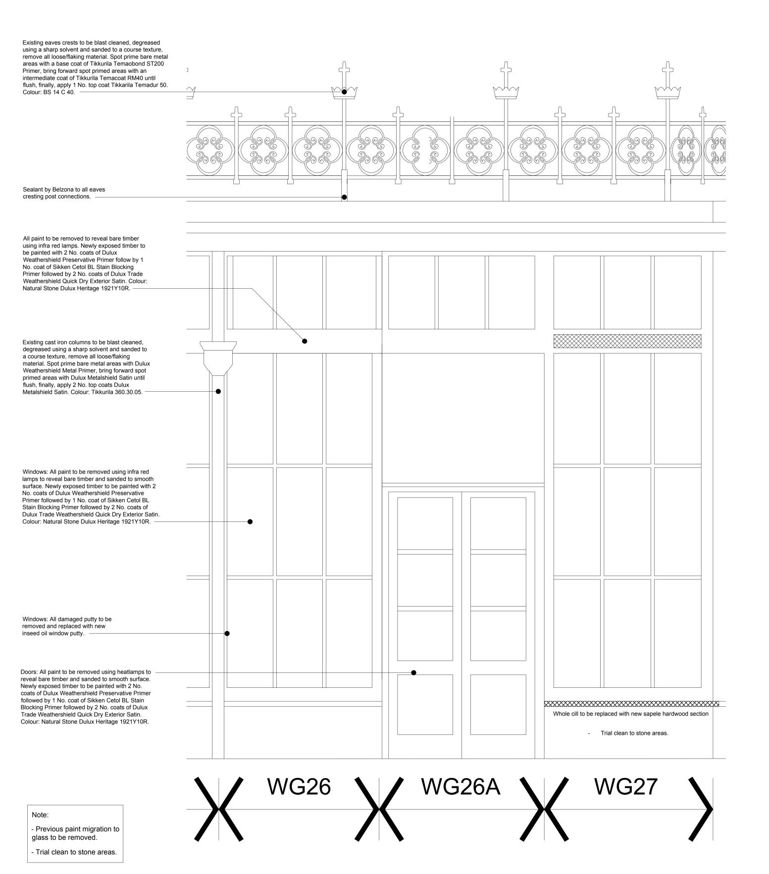
Large Scale Elevation - WG26, WG26A and WG27 Scale 1:20
