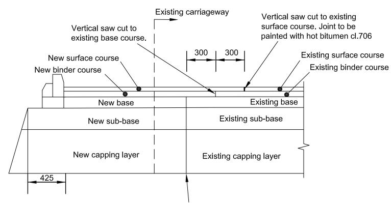
Edge of existing carriageway is to be cut back 300mm to sound face or as instructed by the area Inspector. Tie in extents to be agreed with the area Inspector.
