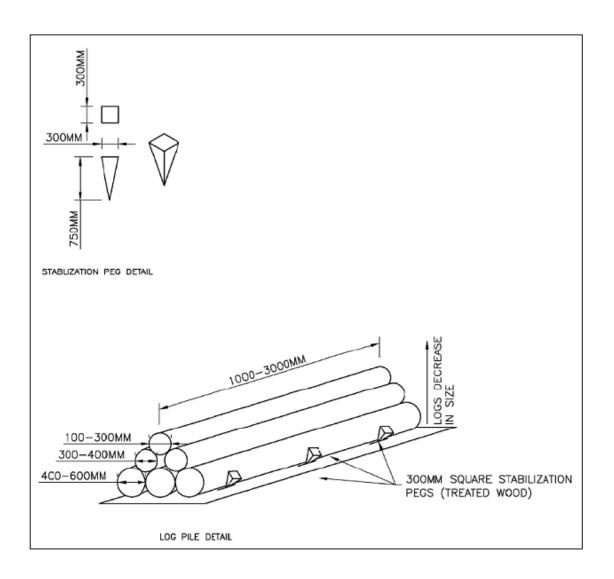
Example of a small, log pile. Additional stability can be provided if needed by hammering posts into the ground at each end of the pile.
