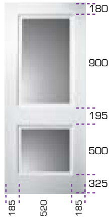
2X66 GLAZED Sash size. MAX 888 x 2098 MIN 710 x 1755 Frame size with Threshold. HxW. MAX 1000 x 2176 MIN 822 x 1833
