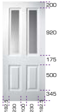
JACOBAN GLAZED Sash size. MAX 888 x 2098 MIN 751 x 1753 Frame size with Threshold. HxW. MAX 1000 x 2176 MIN 863 x 1831
