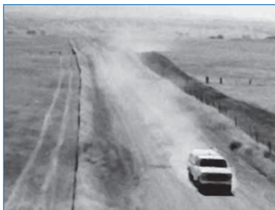
Figure 2.1 Vehicle-raised particles from an unpaved roadway (Source: Midwest Research Institute, USA www.mriresearch.org )
