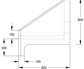
PRE CAST CONCRETE HEADWALL DETAIL
