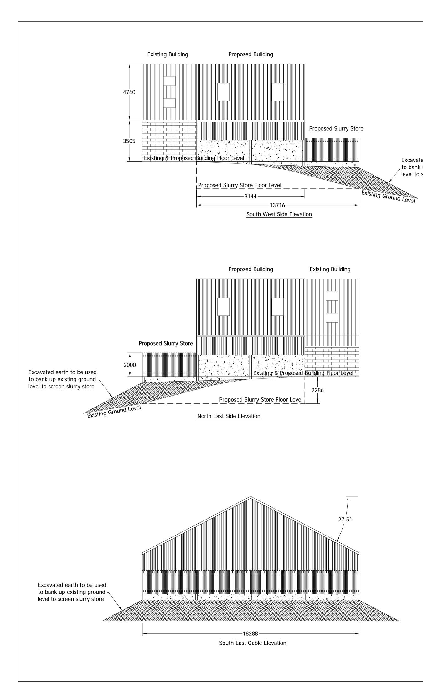
Excavated earth to be used to bank up existing ground level to screen slurry store
