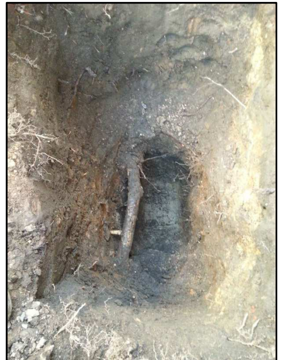
Image 4 – View looking down the trial pit adjacent to Tree 4 at the one 46mm in diameter tree root located near the bottom of the 1m x 1m trial pit
