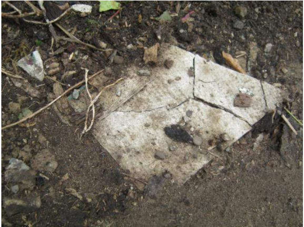
Photo 11: Potentially asbestos containing material
