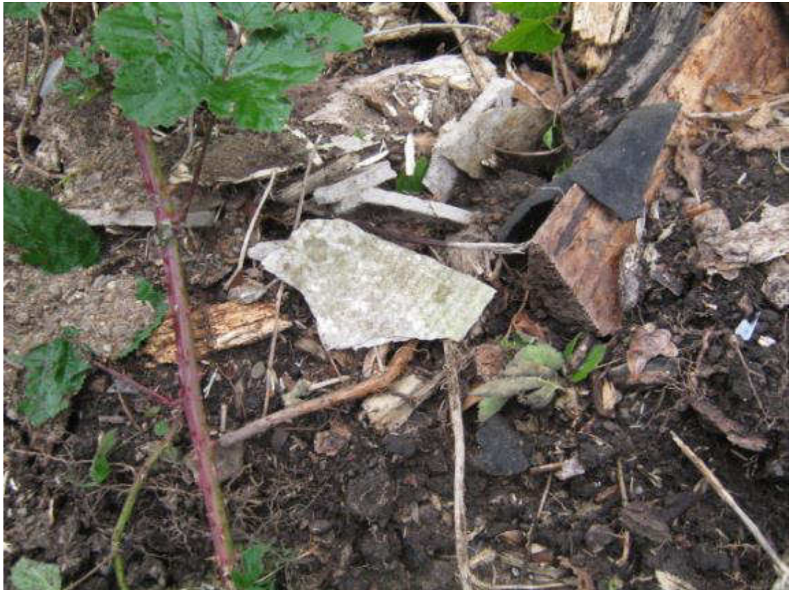
Photo 12: Potentially asbestos containing material
