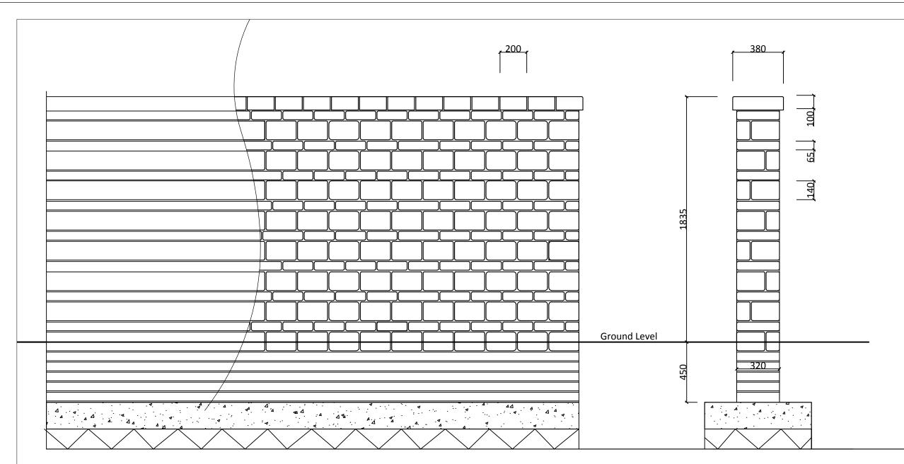
Contractor to accurately measure dimensions & levels on site in order to achieve a satisfactory fit of wall, gates & stepping prior to construction.
