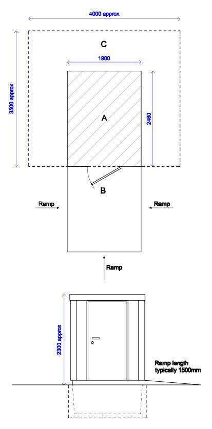
$\frac{KEY}{\text{Hatched area 'A' is building footprint and excevation area. Excevations approx <math>2m \times 2.5m$ . Depth as agreed for each site with Natsol in advance but usually between 750mm and 850mm.
