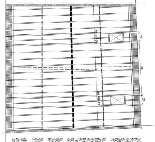
ALLOW FOR NEW RAFTERS TO THE REAR (AS A MINIMUM PROVISION) AND TIMBER TREATMENT THROUGHOUT. ALL ROOF COVERINGS ARE TO BE REMOVED AS ARE ALL BATTENS. ALLOW FOR 70% RECLAIM AND ALL NEW SPARS. ROOF TO BE INSULATED WITH 100mm KINGSPAN BETWEEN RAFTER LINE AND UNDERDRAWN WITH 50 BELOW. ÀBOVE AND BELOW). ALLOW FULL VENTILATION SOFFIT AND RIDGE. TYVEK MEMBRANE. OR EQUIVALENT U VALUE WITH 50 SUPERQUILT)
