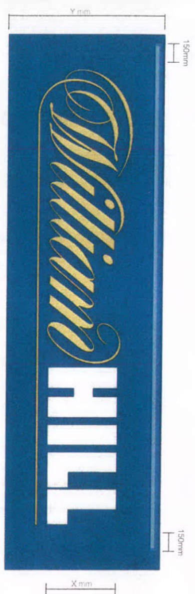
Item EXF 01 Folded aluminium fascia sign powder coated blue with vinyl logo and trough light to illuminate. 300mm longer than logo Scale 1:20
