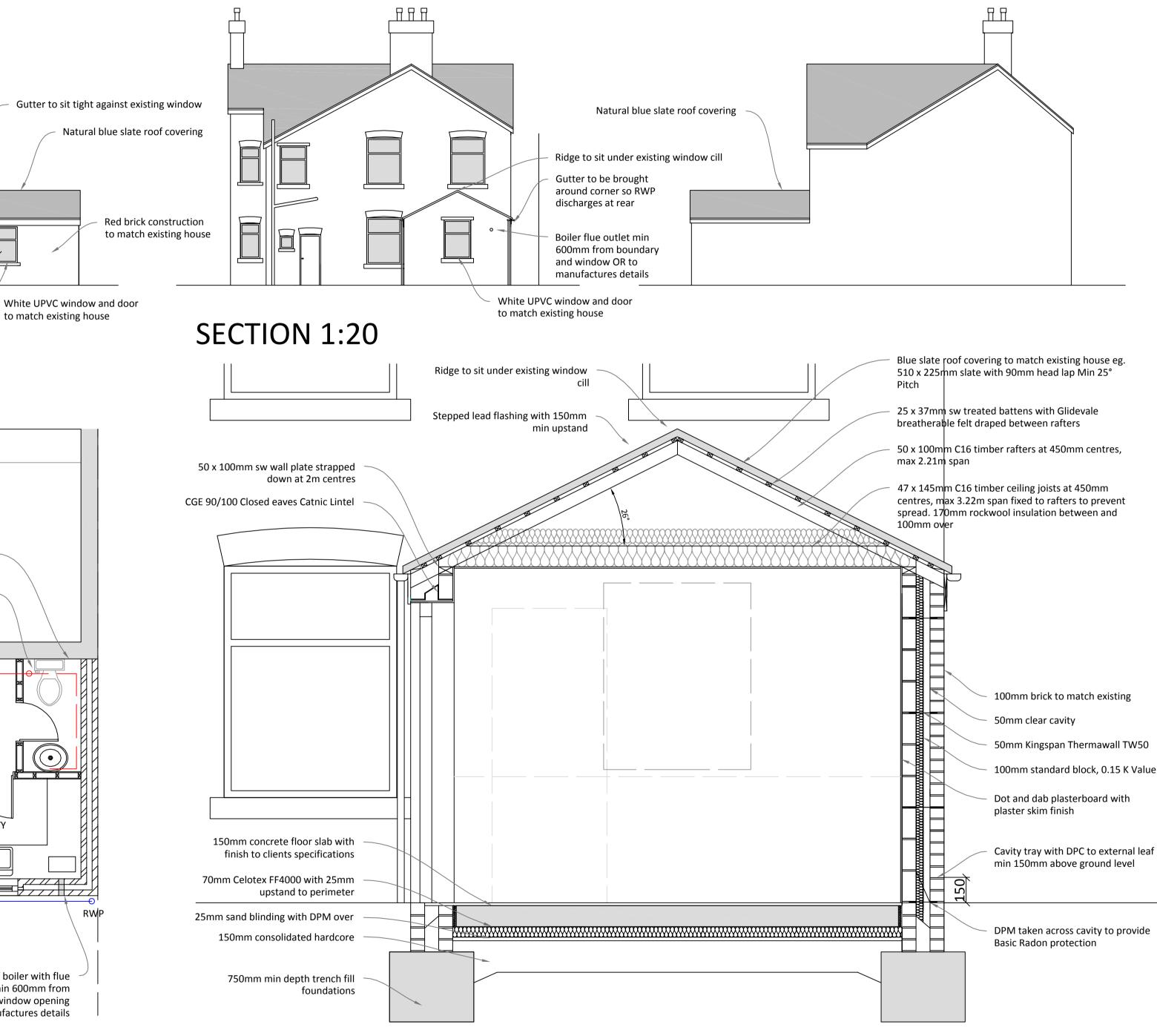
All walls constructed using stainless steel vertical twist type retaining wall ties built in at 750mm ctrs horizontally, 450mm vertically and 225mm ctrs at reveals and corners in staggered rows. Wall ties to be suitable for cavity width and in accordance with BS 5268-6.1: 1996 and BS EN 845-1: 2003
