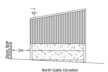
Roof sheeting to be factory coated coloured fibre cement sheeting coloured Juniper Green (12B29). Vertical cladding to be treated Yorkshire boarding. Below cladding to be pre-stressed concrete panels. All dimensions are stated in mm
